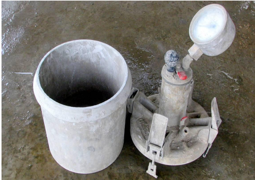
Figure 1: Air Content Pressurized Air Pot Apparatus
